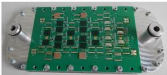
Figure 5. Inverter single phase prototype
